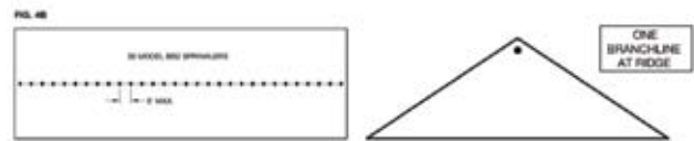
ATTIC SPRINKLER LAYOUT
