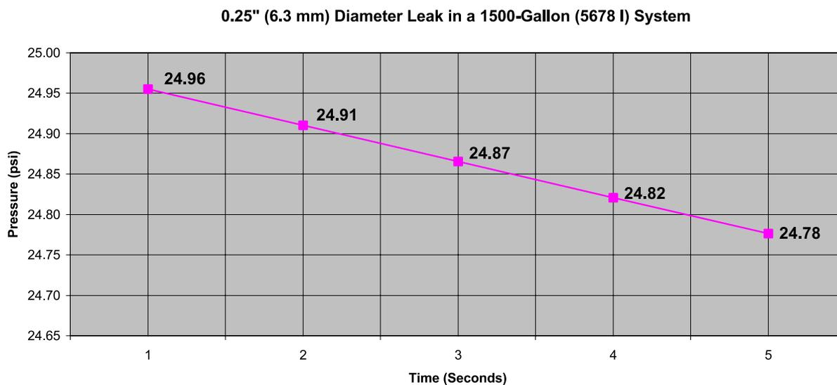
**Figure 8- Air Leak Curve -Detail**
