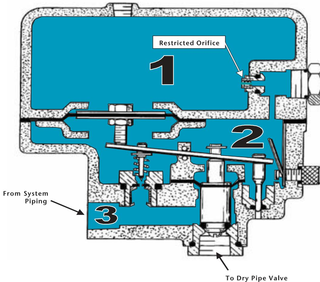
**Figure 3 - Section View of a Mechanical Accelerator**
