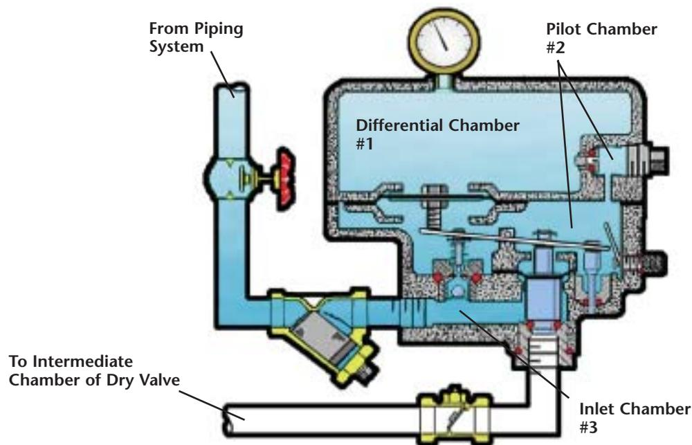
**Figure 2 - Tyco ACC-1 Accelerator as Installed in the Set Position**
