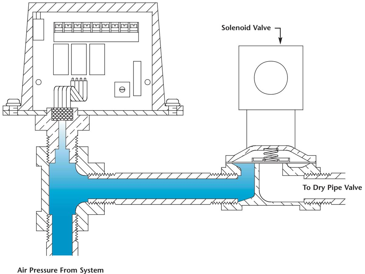
**Figure 10 - QRS Switch and Solenoid Valve in the Set Position**
