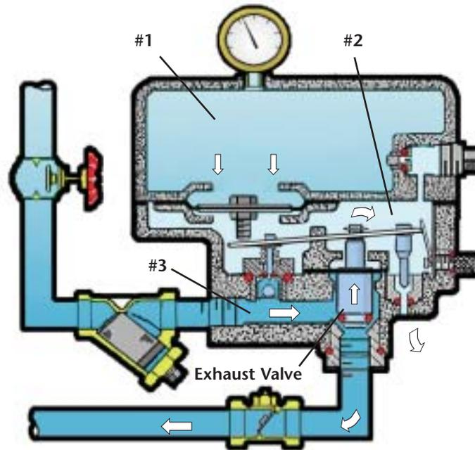
**Figure 6 - Upon 2 psi Differential Pressure (Chamber 1 & 2) - Accelerator Trips**
