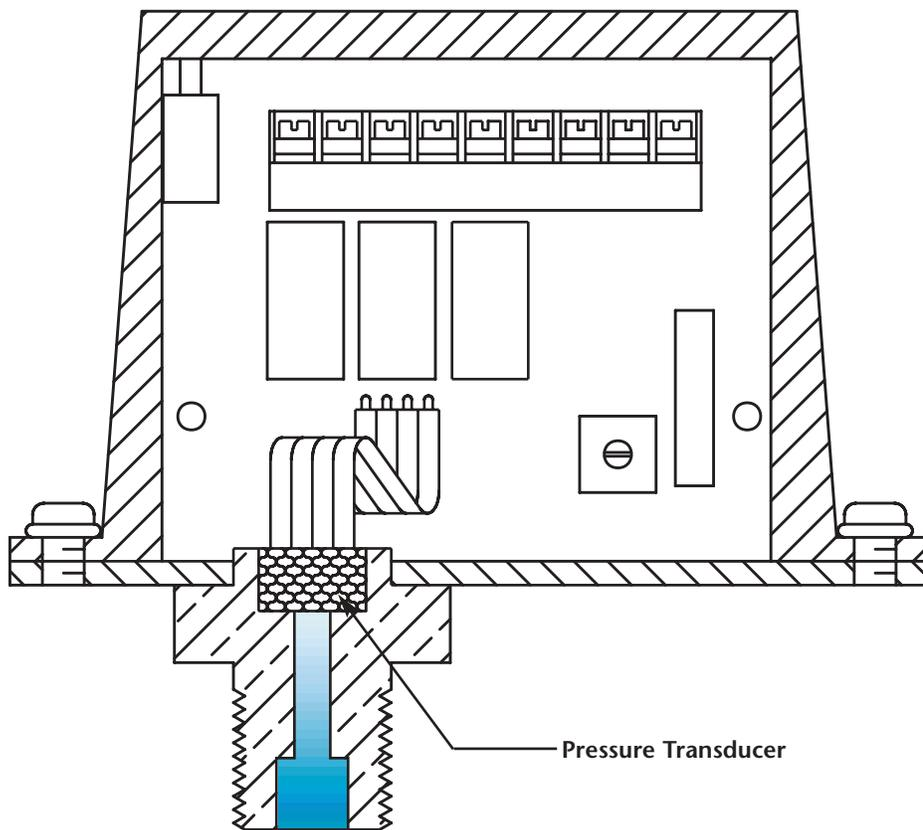
Figure 9 - Section of QRS Switch
