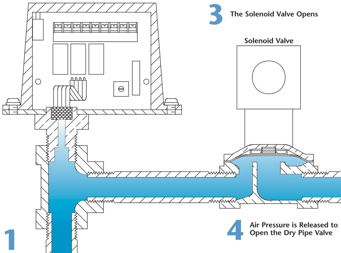
**1** As Air Pressure Drops Due to Sprinkler Activation
