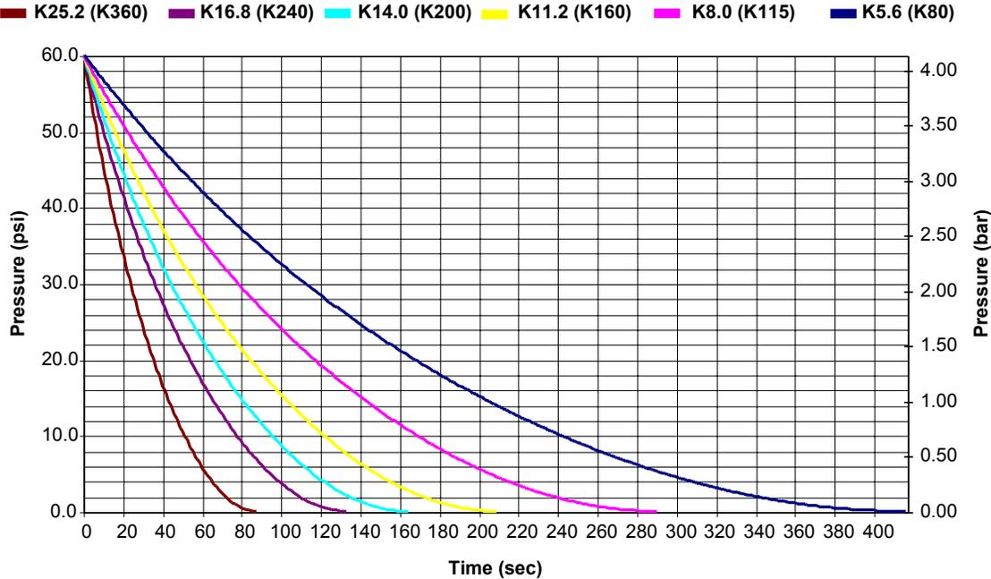
Figure 3 - The Effect of Test Orifice Size on the Rate of Pressure Drop in a Dry System
