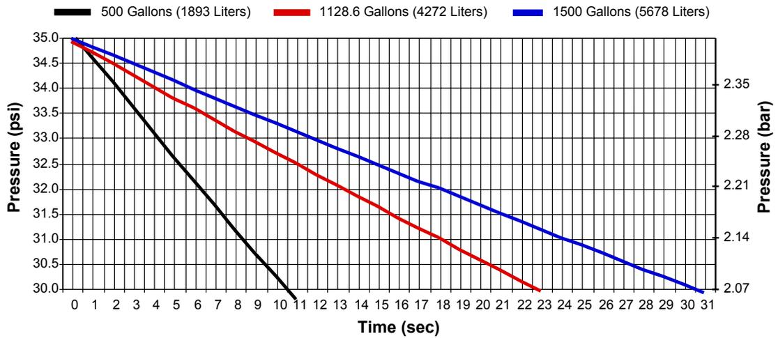
*Figure 1 - Air pressure vs. Time for 35-psi to 25-psi (2,4 to 1,7 bar) Pressure Drop through a K5.6 (K80) sprinkler*
