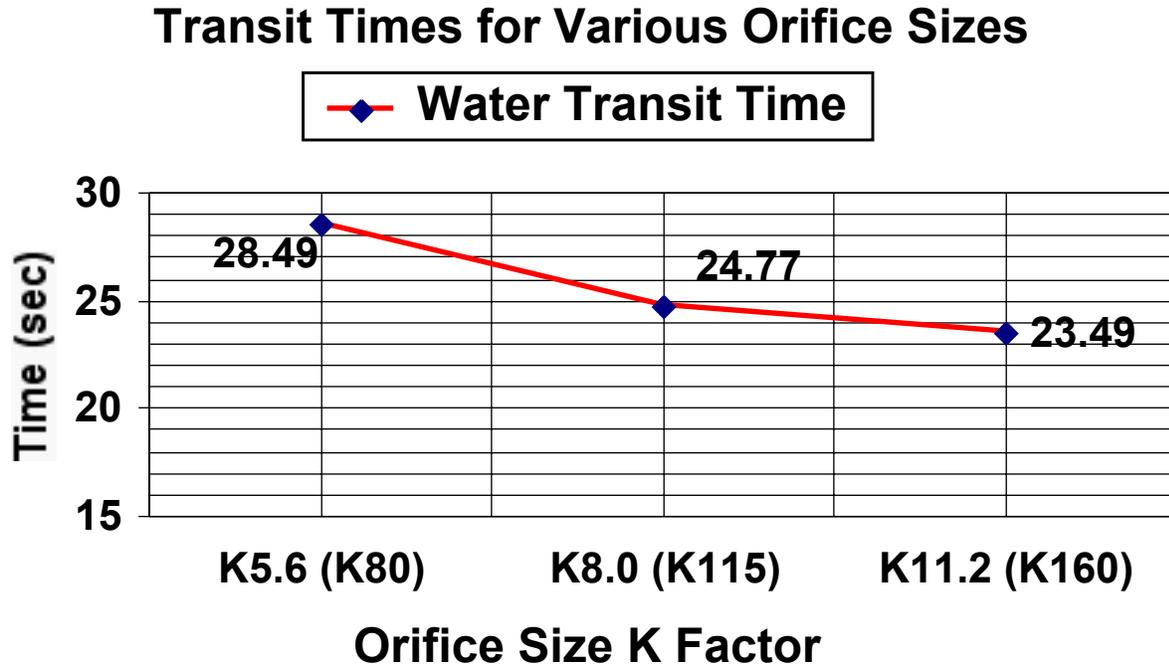
*Figure 5 - Comparison of a single K5.6, K8.0 and K11.2 (K80, K115 and K160) water transition times.*
