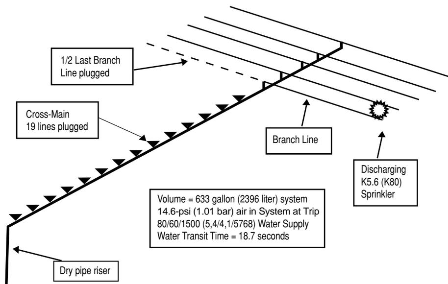
**Figure 12 - Isometric of a single branch line tee (Figure 11) with 4 additional branch lines beyond the Inspectors test valve.**
