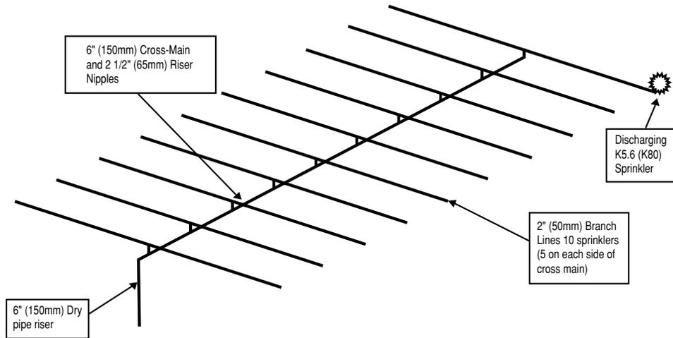
**Figure 9 - Isometric of a center feed tree - 410.8 gallon (1555 liter) capacity (10 lines by 10 lines sprinklers)**
