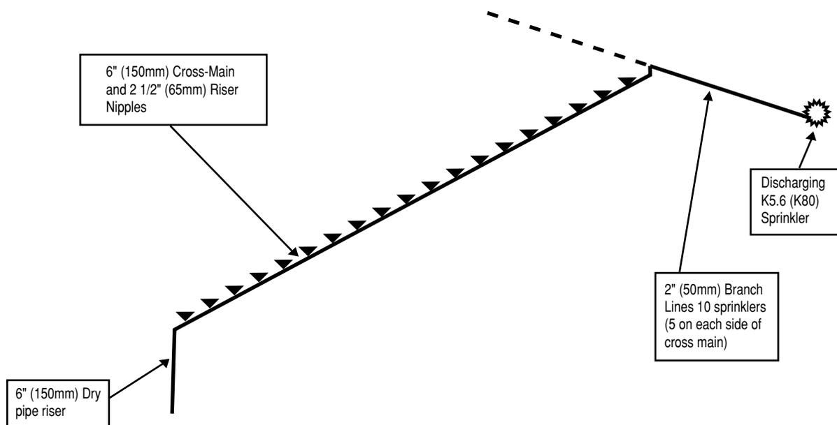
**Figure 11 - Isometric of a single branch line tree - (same systems as Figure 4 with exceptions noted)**
