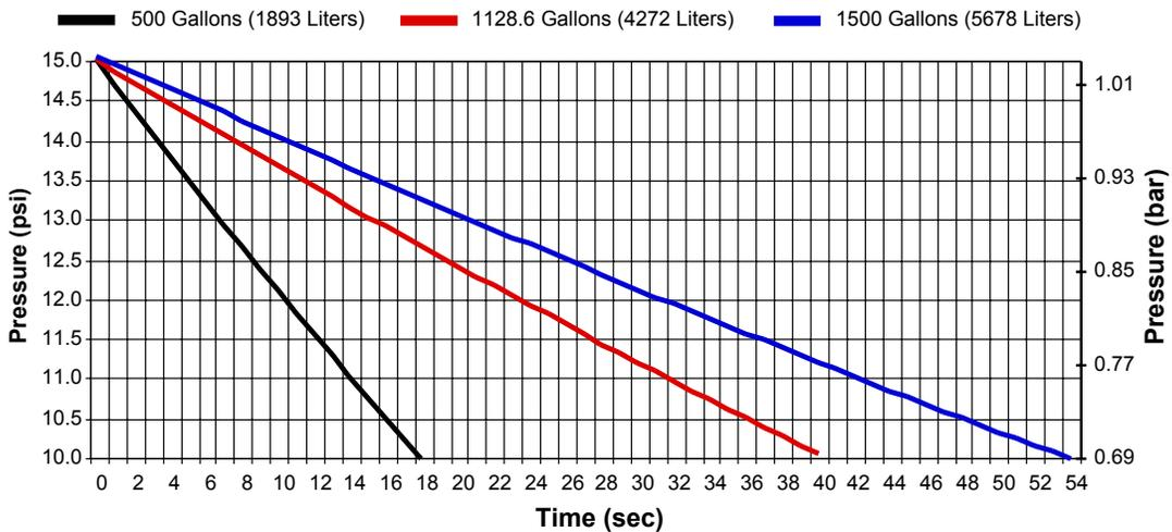
*Figure 2 - - Air pressure vs. Time for 15-psi to 10-psi (0,1 to 0,7 bar) Pressure Drop through a K5.6 (K80) sprinkler*
