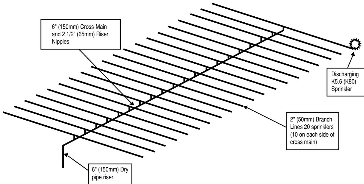
**Figure 4 - 1128.6 gallon dry pipe system**
