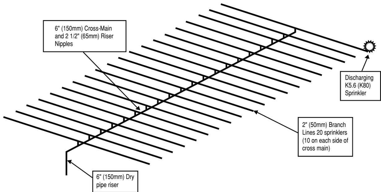
**Figure 8 - Isometric of center feed tree - 1128.6 gallon (4272 liter) capacity
