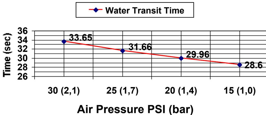
Figure 7 – Comparison water transition times with different air pressures in the system.
