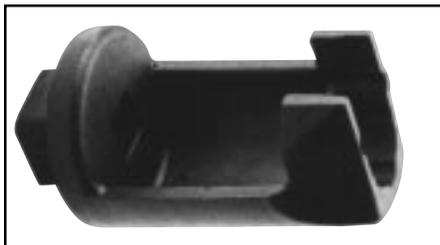
obtained by applying the sprinkler head wrench and turning either clockwise or counterclockwise. Note that no locking is required when the sprinkler is in its desired position.
