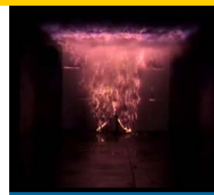
45 Seconds—Near Flash Over Conditions
