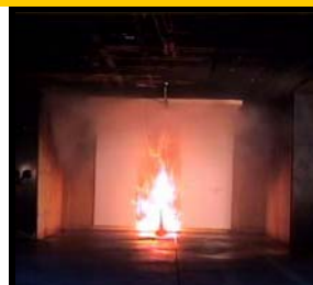
22 Seconds— Sprinkler Operates
