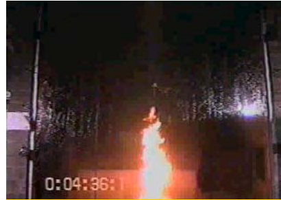
40 kW Fire Test
